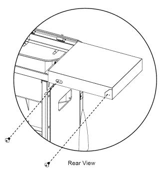
15. To begin installation be sure to align large shelf (holes) with the small holes in the shelf bracket assembly. Insert (2)  $\#10 \times 1/2$ " Truss head screws (phillips drive) into largest hole on outside rear corner of shelf carefully aligning with small hole in shelf mounting bracket. Repeat procedure for inside rear.
